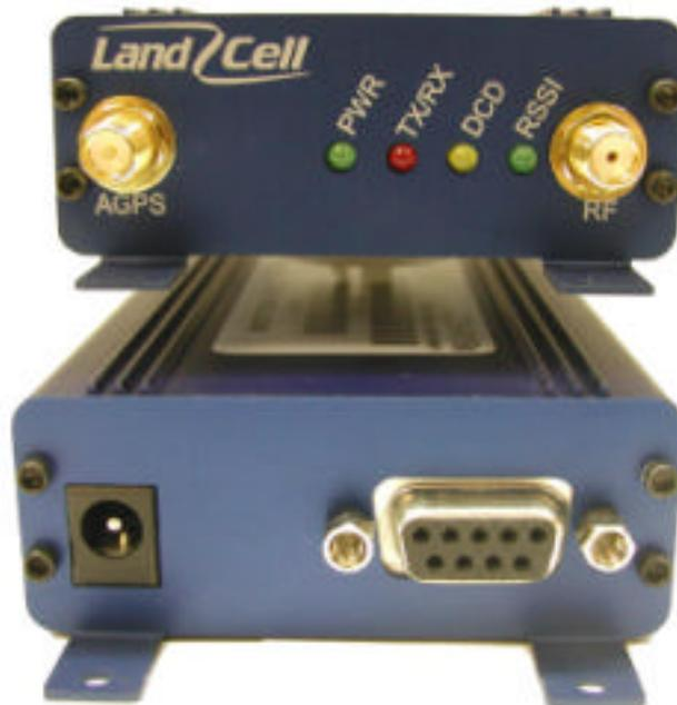
The lower modem in the image above depicts the rear side of the modem. The rectangle on the left side is the location of the DC power supply barrel jack connector. On the right side is the female DE-9S serial connector.
