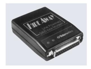
The HA2400LP is designed for those applications where no external source of power is available. The HideAway derives its power from two isolated sources: Power from the RS232 interface (TXD, RTS & DTR) activates the HideAway's RS232 drivers, the AT Command set controller and the optical relay that picks up the telephone line; Power from the telephone line then activates the data pump and ancillary telephone line components.
